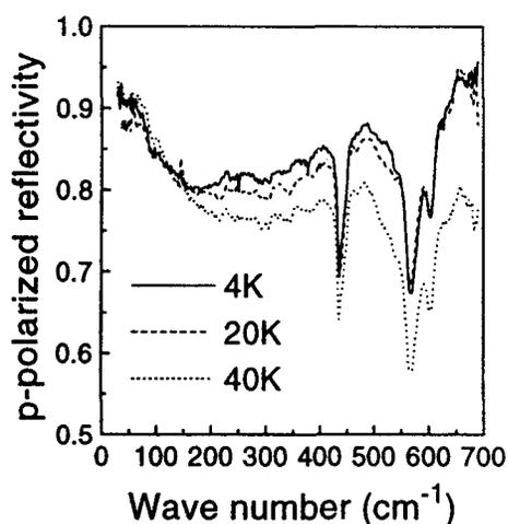
Figure 1. Grazing-incidence  $p$ -polarized reflectivity  $R_p$  of a superconducting  $\text{Sm}_{2-x}\text{Ce}_x\text{CuO}_{4-\delta}$  crystal at 4, 20, and 40 K.
