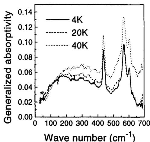
Figure 2. Generalized absorptivity calculated from  $R_p$  of  $\text{Sm}_{2-x}\text{Ce}_x\text{CuO}_{4-\delta}$  at 4, 20, and 40 K.
